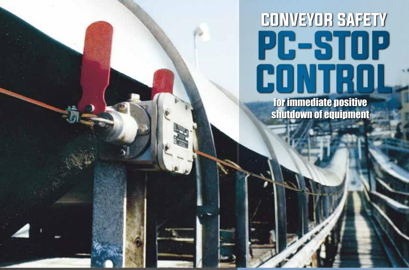
The PC Stop Control can be used for emergency shutdown of conveyor systems, elevator equipment, bulk handling systems, cranes, production and assembly lines, or any other equipment which may require immediate, positive shutdown.
